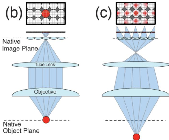
Figure 5: (b), (c) The red point stands for a point source generating illumination. Red regions on top shows the intensity of illumination arriving at the sensor plane[3].
