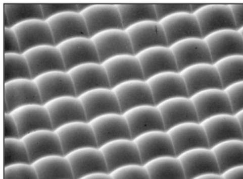
Figure 3: Microlens array[1]
