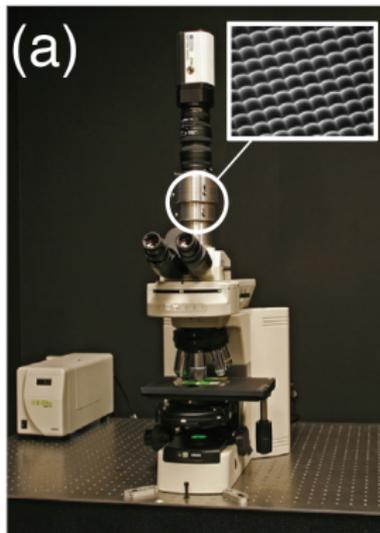
Figure 2: (a) A microscope with a microlens array[3]
