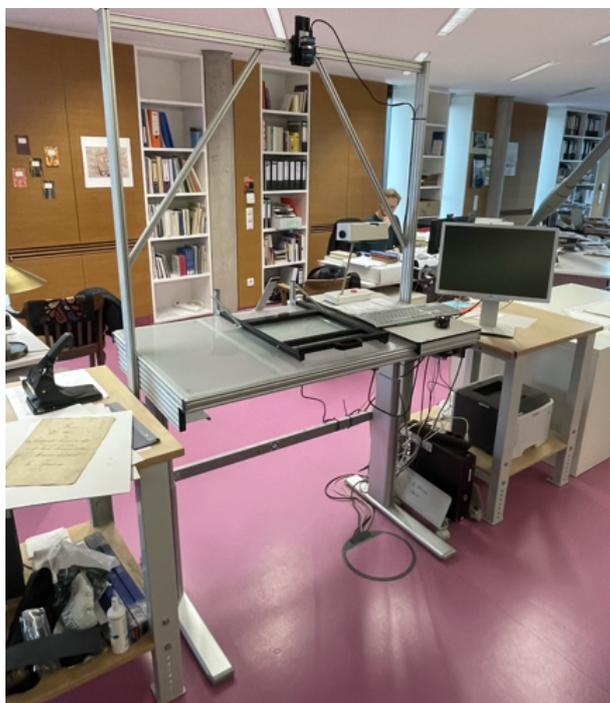
Figure A.3: Set up for digitization of the watermark dataset at DNB in Leipzig
