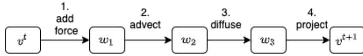
Figure 10: Computational steps in the stable fluid scheme [19] for advancing the flow field to the next time step 1.) External forces are applied as \mathbf{w}_1 = \mathbf{v}^t + \Delta t \mathbf{f} . For our purposes, the residual correction model is applied in this step 2.) The advection of the fluid by itself is calculated by the method of characteristics [19] 3.) The effect of diffusion is taken into account by solving an implicit form of the diffusion equation. The \Phi_{Flow} implementation deviates at this point by explicitly computing the vector Laplacian by finite-difference discretization. Our effective viscosity model comes in here. 4.) \mathbf{w}_3 is projected onto the space of divergence free fields by solving the associated Poisson problem.
