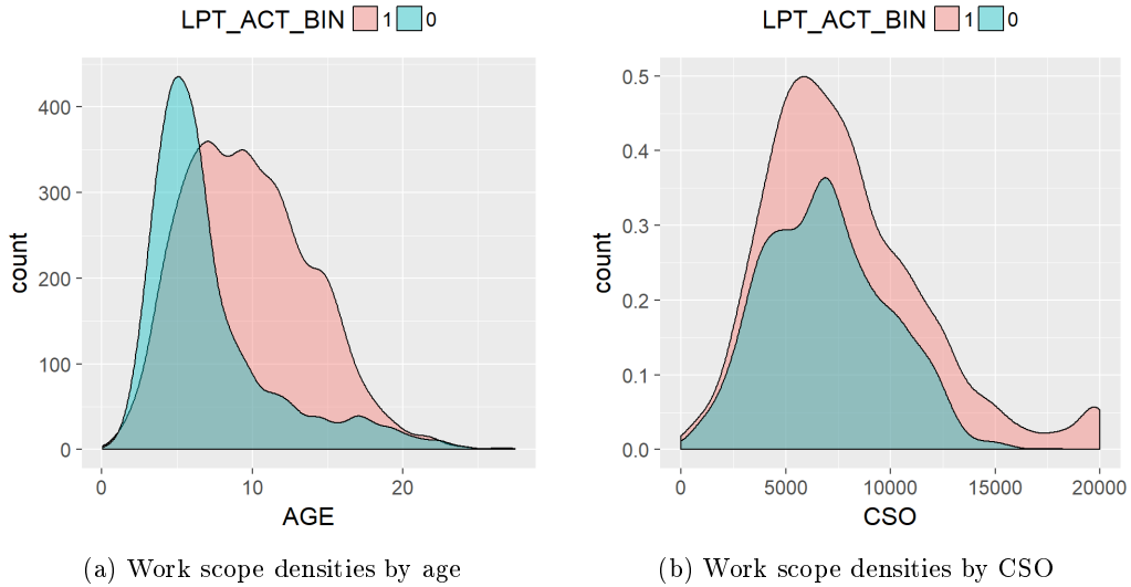
Figure 4.4: This plot shows density estimates for exposed and non-exposed shop visits by age (left) and CSO (right). The exposure rate is highest for engines between 7 and 20 years of age. Furthermore, runs with a length of 7000 or above 17000 cycles can expect a high exposure rate
