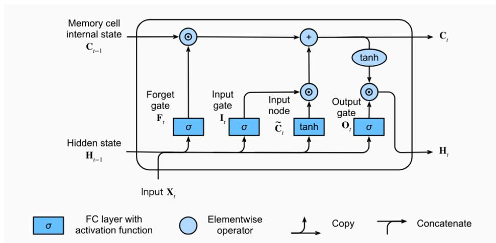
Figure 1: LSTM cell graphical illustration of data flow. [2]
