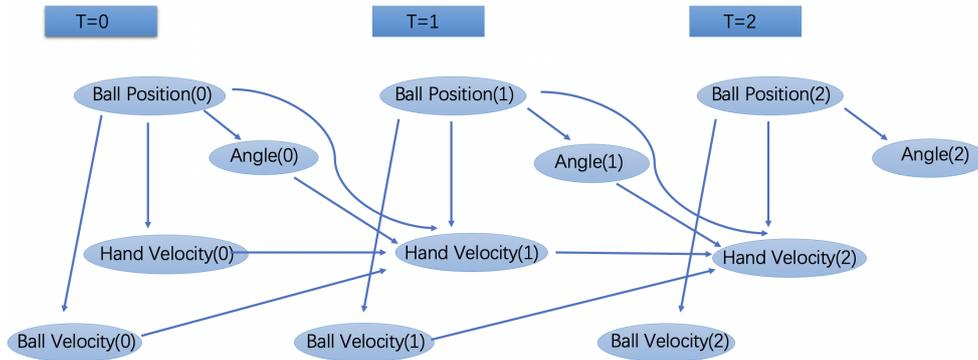
Figure 4: DBN model without haptic feedback
