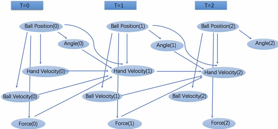
Figure 3: DBN model with haptic feedback
