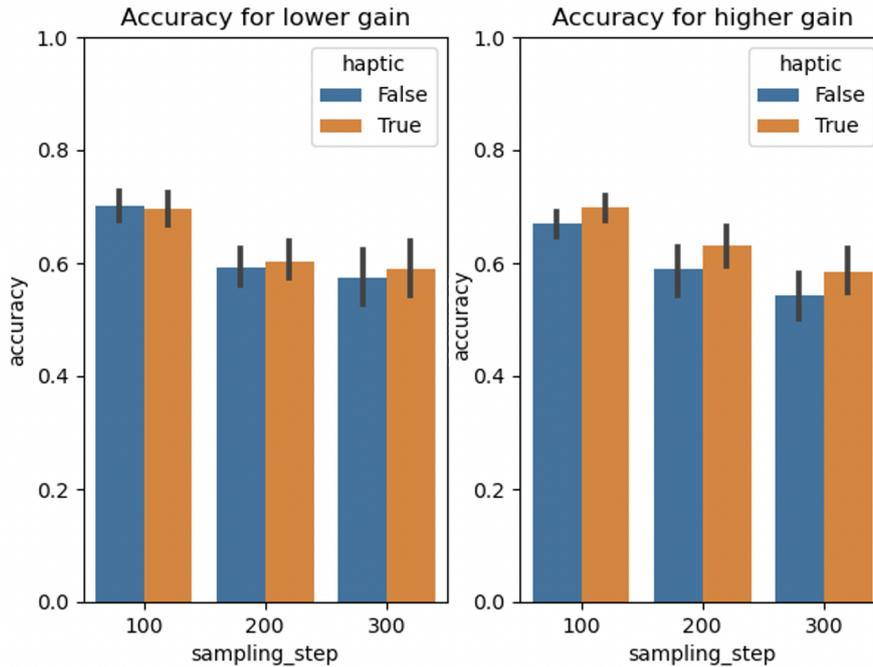
Figure 11: The accuracy of DBN with reduced nodes. Blue bars shows the DBN with two nodes: hand velocity, ball relative position. Orange bars shows the DBN with three nodes: hand velocity, ball relative position and force feedback.
