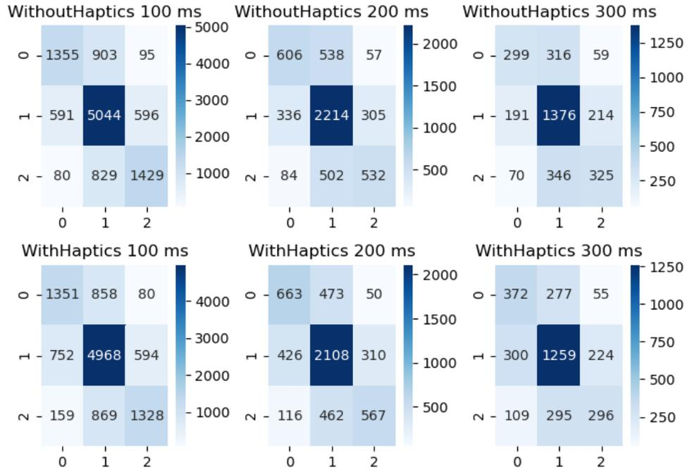
Figure 9: Confusion matrix for DBN model. Here the x-axis is the actual state and the y-axis is the predicted state. 0 means down, 1 means still, 2 means up
