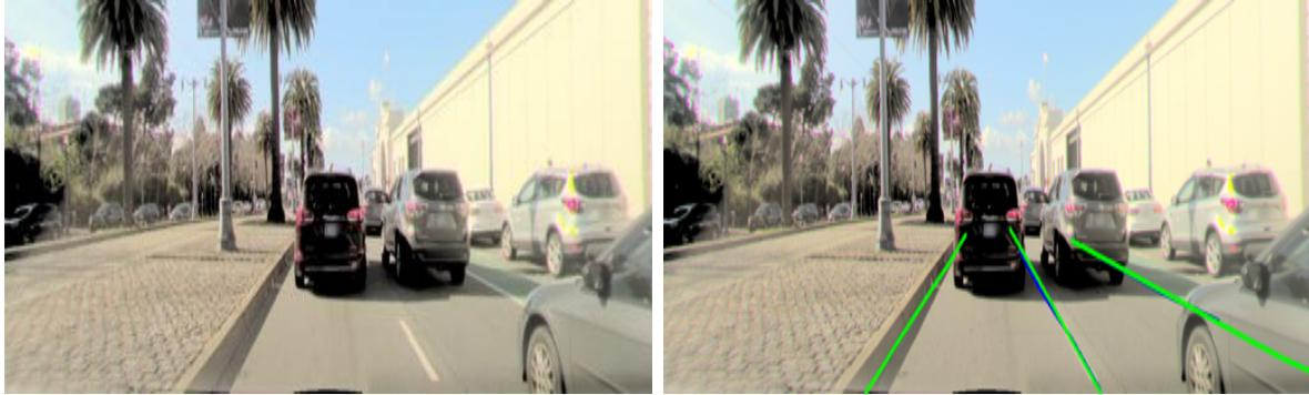
Figure 17: Performance of LaneATT on an image from the BOSCH dataset. (Left): unannotated image, (Right): annotated image. Green lines are network predictions, and blue ones are ground truth annotations.
