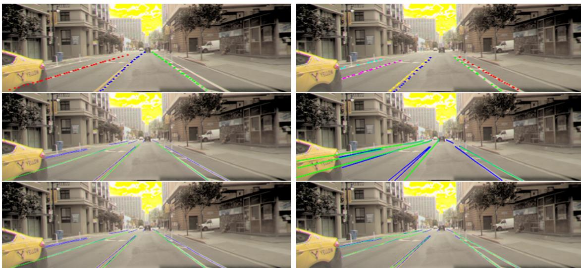
Figure 25: (Top to bottom) Overfitting experiments on PINet, LaneATT and LaneAF, (Left): Before overfitting, (Right): After Overfitting
